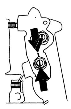
The distinguishing feature of the various shut-off devices is the shape of the stop/regulating lever.
